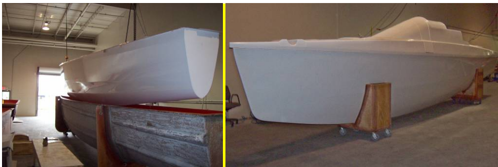
One of the hulls of G-Force 36 is removed from its mold.
